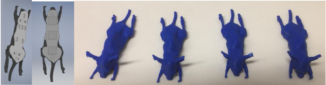
Figure 15. (Top row) the CAD design of the mouse-mimicking phantom. The first version is for embedded TLD-100 chips and the second version is for embedded OSLD chips. (Bottom row) the actual 3D printed phantoms based on the CAD design. The weight of the phantom is 24.5 \pm 0.1\text{g} .
